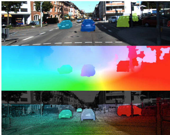
Figure 3.11: Estimated moving object, optical flow and scene flow [29], used with permission.
